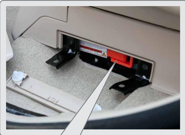
Wearing insulated gloves, pull the lever (do not slide) and remove the service plug grip.
